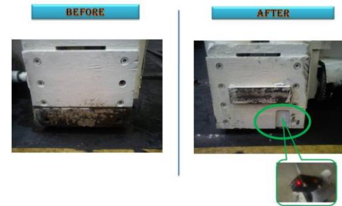
Figure 11: Manual (Before) and Automated (After) Moving Blaster
