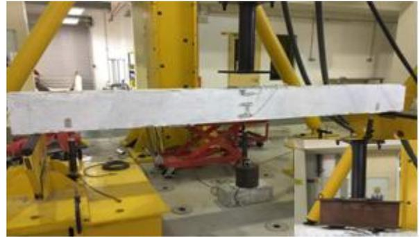
**Plate1:** Simply Supported Beams under Fatigue loading.
