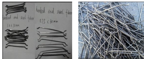
Figure 1: Hooked end steel fibers
