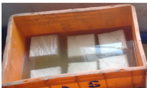
Figure 11: Curing of Cubes in H_2SO_4
