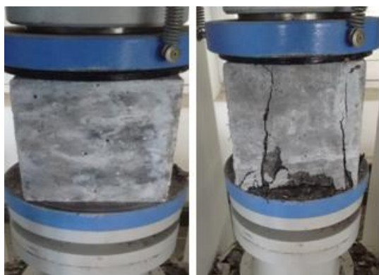
Figure 2: Compression testing of cube
