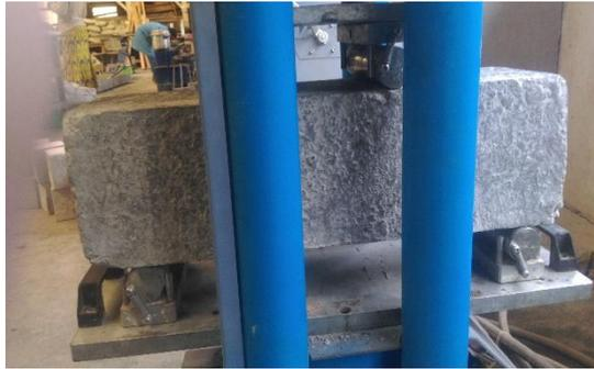
**Figure 2:** Flexural strength test
