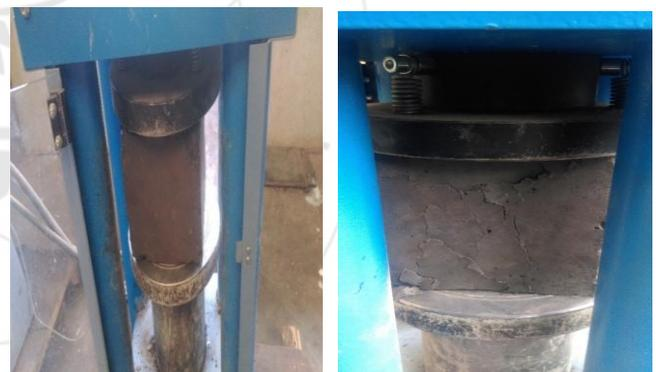
a) Cube placing before testing      b) Cube after testing
