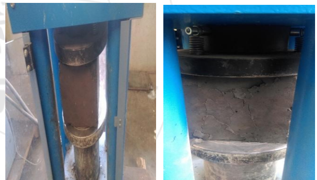
Figure 4: Compressive strength test
