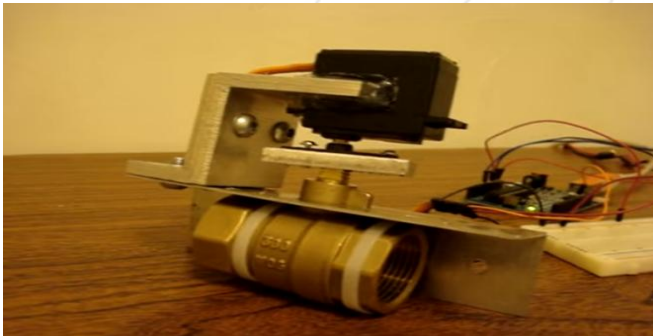
Figure 7: T-type valve with servo motor
