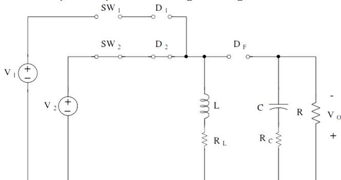
Figure 3: Mode 2, SW<sub>2</sub> and D<sub>2</sub> conduct, SW<sub>1</sub> off
