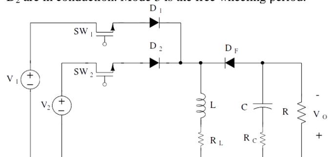
**Figure 1:** Dual input Buck Boost Converter
