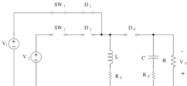
Figure 2: Mode 1, SW<sub>1</sub> and D<sub>1</sub> conduct, SW<sub>2</sub> Off
