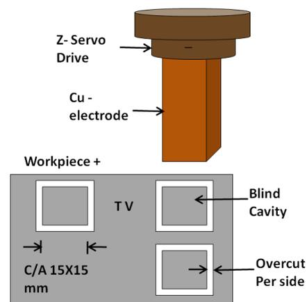
Figure 1: EDM process with overcut per side
