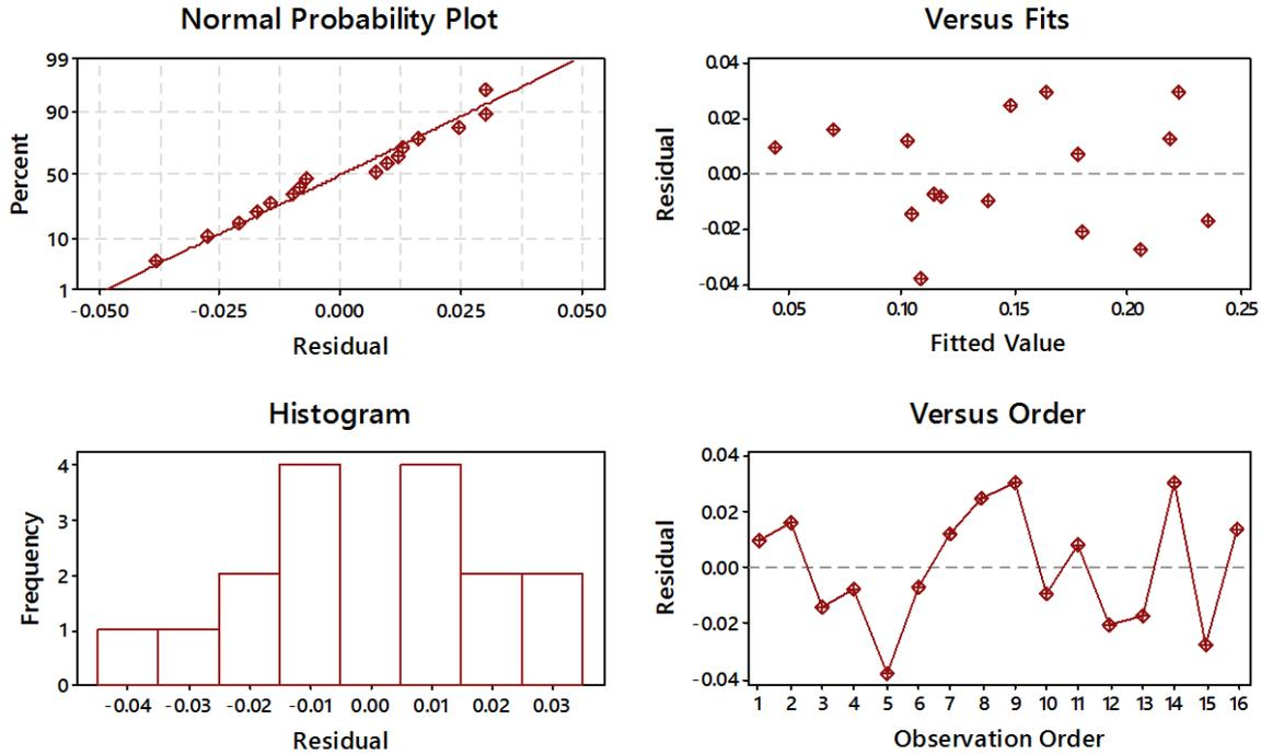
**Figure 3:** Residual plot analysis for overcut per side
