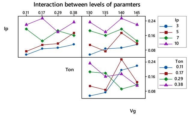
**Figure 6:** Interaction plot for overcut per side
