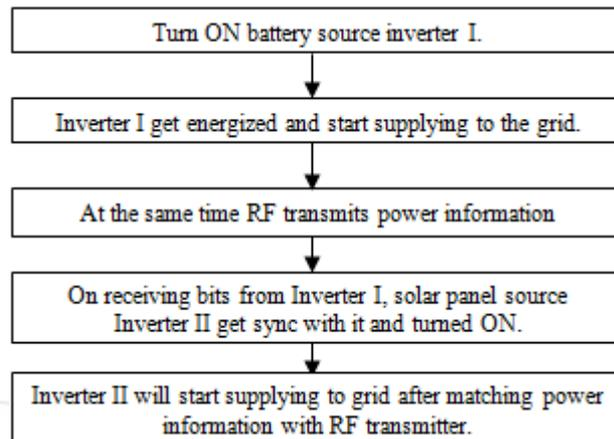
**Figure 7:** Flowchart showing working of proposed system
