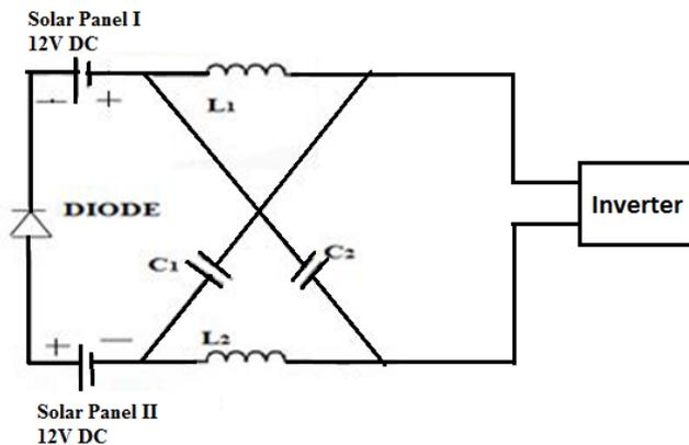
**Figure 5:** Schematic diagram of E-Z source
