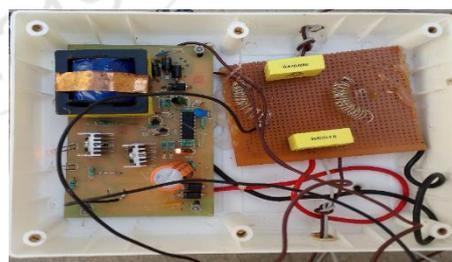
**Figure 9:** PCB of Inverter II with EZ source
