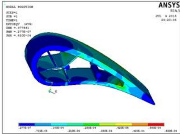
**Figure 11:** Strain Analysis on Guide Vane with Impingement Cooling Design
