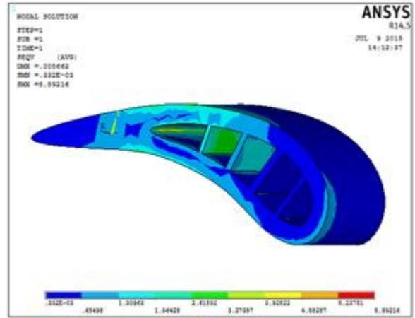
**Figure 8:** Stress Analysis on Guide Vane with Impingement Cooling Design
