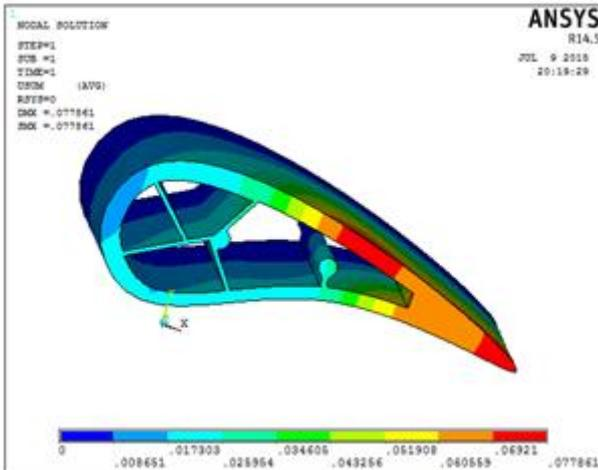
**Figure 7:** Displacement Analysis on Guide Vane with Showerhead Cooling Design
