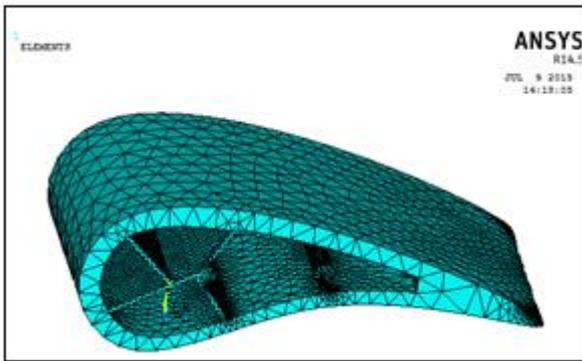
**Figure 5:** 3D Meshed model of Guide Vane with Showerhead Cooling Design
