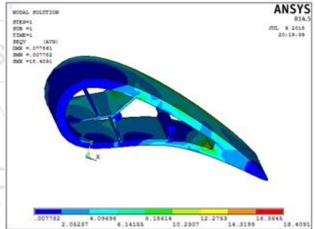
**Figure 9:** Stress Analysis on Guide Vane with Showerhead Cooling Design
