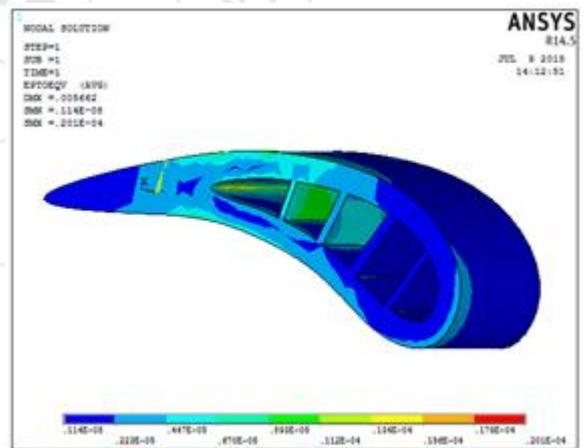
**Figure 10:** Strain Analysis on Guide Vane with Impingement Cooling Design
