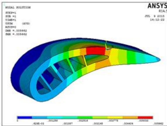
**Figure 6:** Displacement Analysis on Guide Vane with Impingement Cooling Design
