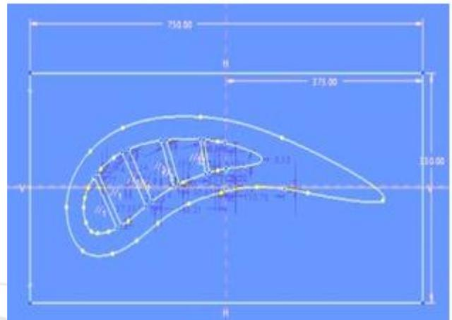
**Figure 2:** Profile and Dimensions of Guide Vane with Impingement Cooling Design
