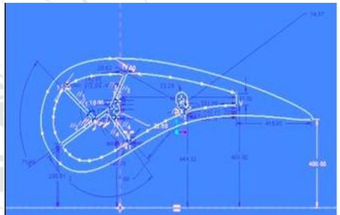
**Figure 3:** Profile and Dimensions of Guide Vane with Showerhead Cooling Design
