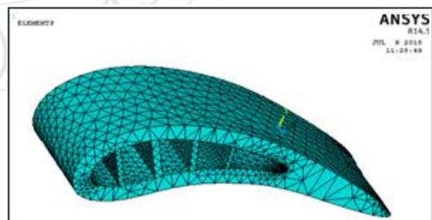
**Figure 4:** 3D Meshed model of Guide Vane with Impingement Cooling Design
