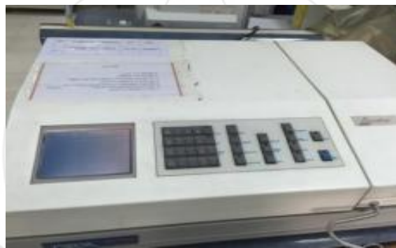
Figure 3: UV spectrophotometer (Cecil 7200, England) used in the study
