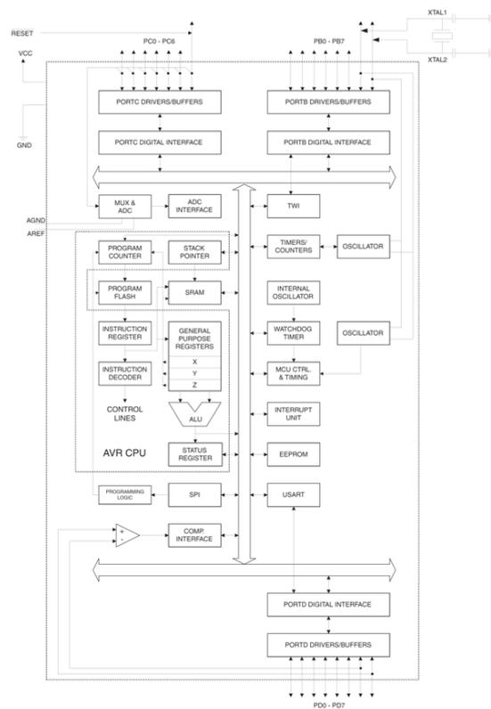
**Figure 2:** Block diagram ATmega8
