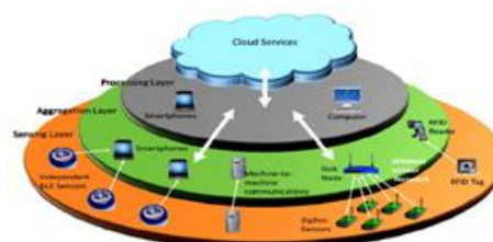
Figure 1.1: Architecture of an IoT [3]
