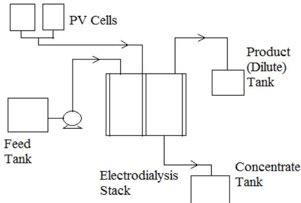
**Figure 8:** Solar Electro-dialysis System
