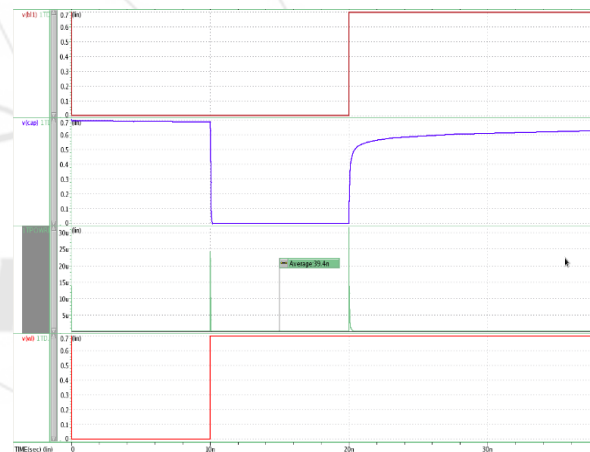
Figure 20: Read cycle of 1T1C DRAM cell
