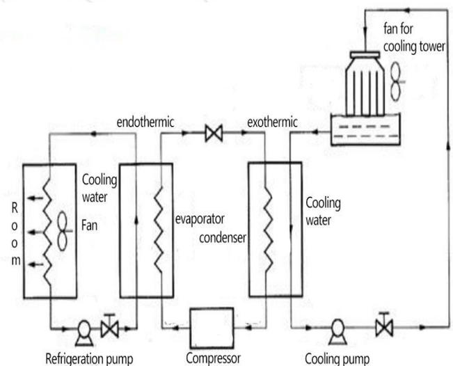
**Figure 1:** The composition of central air conditioning system
