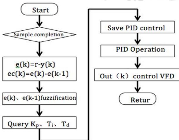
**Figure 3:** Fuzzy PD algorithm routine flowchart cooling pump
