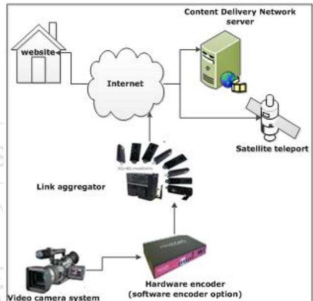
Figure 1: Block diagram of a link aggregator
