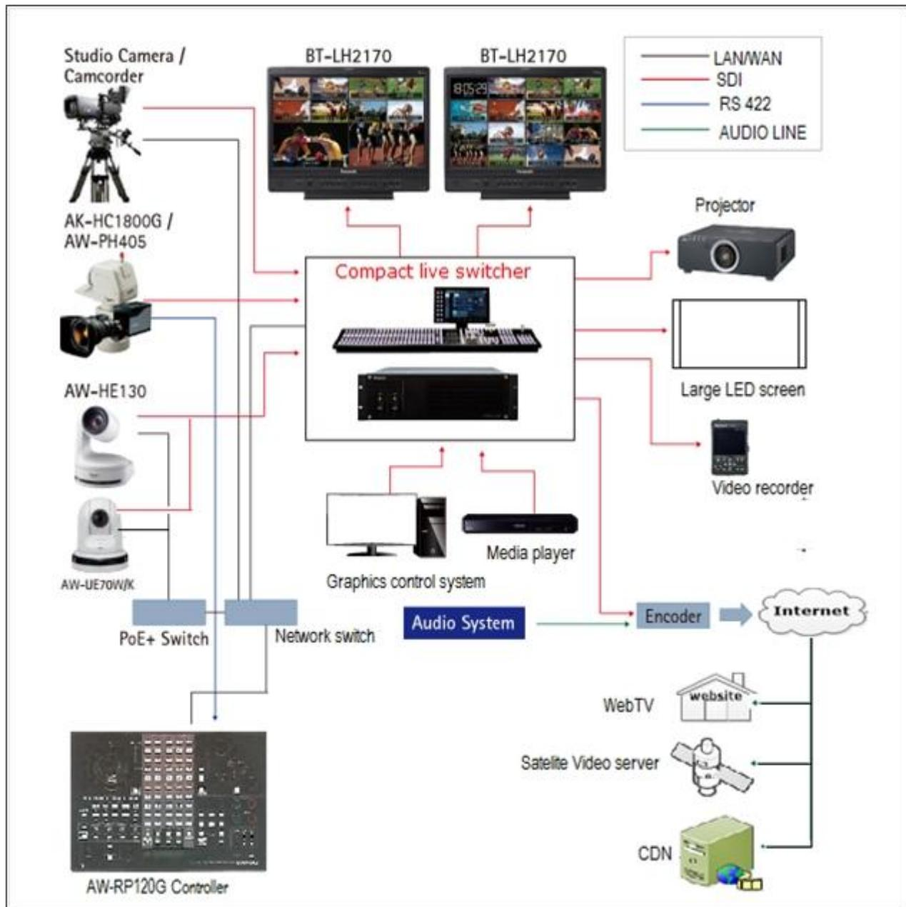
Figure 4: Schematic of an Integrated Remote-controlled HD camera system in operation at the central location
