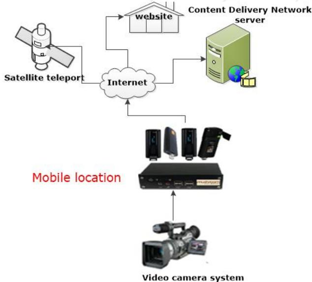
**Figure 3:** Block diagram of an „on the go“ implementation of a non-localized event
