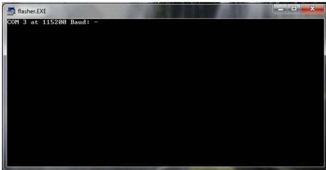
Select the baud rate to 115200 and the COM port. Locate the HEX file and press the flash button. It will initiate the port. Connect the Axon microcontroller using USB cable and switch on the microcontroller power. The file will be transferred to the microcontroller memory.
