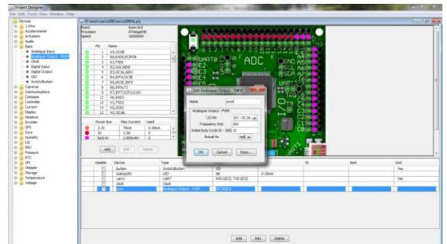
Name the device and give the initial values. After adding the all devices save the file and select tools menu to generate the project file. Enable create the avrstudio project file, locate where the Webbotlib is installed and set the path where the generated files to be stored. A project file will be created.
