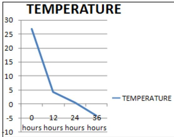
Figure 10: By using D.C compressor Time required to cool the load =36 hours
