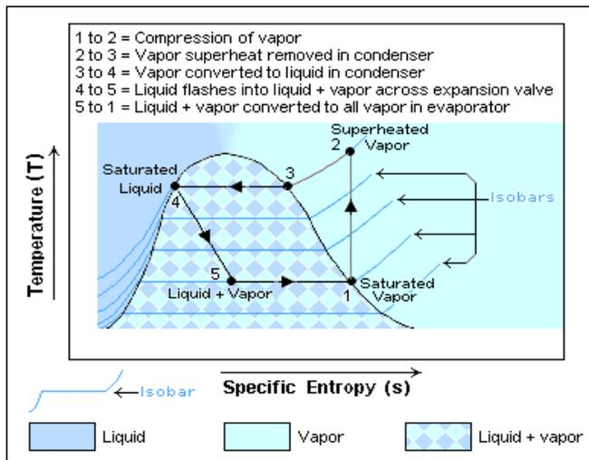
**Figure 1: Thermodynamic Cycle (T-S Diagram)**
