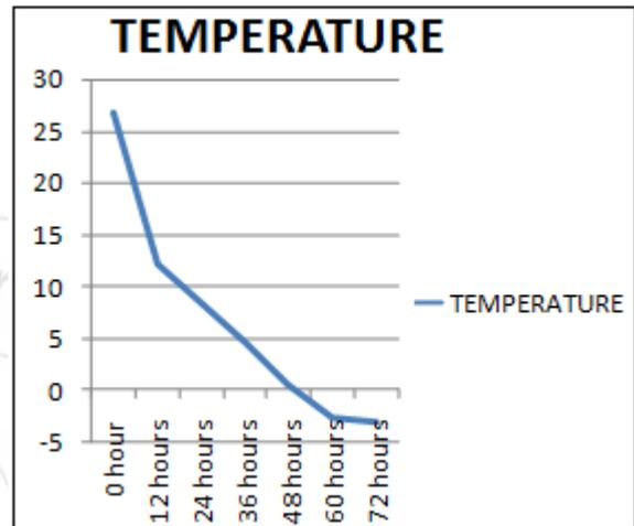
Figure 12: By using D.C compressor time required to cool the load =72 hours
