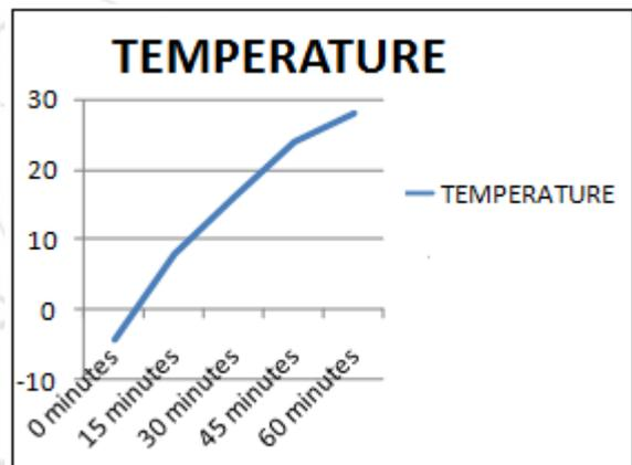
Figure 9: In warm up cycle initially having  $-4.3^{\circ}\text{C}$  without phase change materials it reaches  $28^{\circ}\text{C}$  within 60min.
