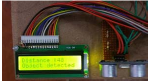
Figure 16: On detecting the object at the front end of the vehicle the message is displayed on LCD
