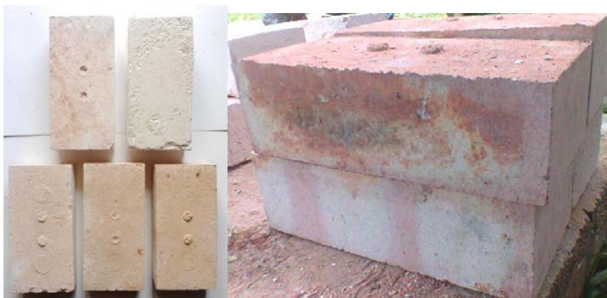
Rice husk insulating fired bricks
