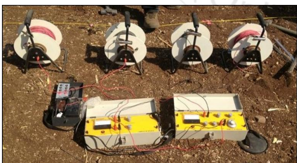
Image 5.1: Photo showing connection for resistivity method
