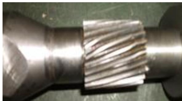
**Figure 1:** The gear after failure
