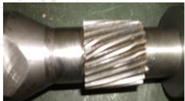
Figure 1: The gear after failure
