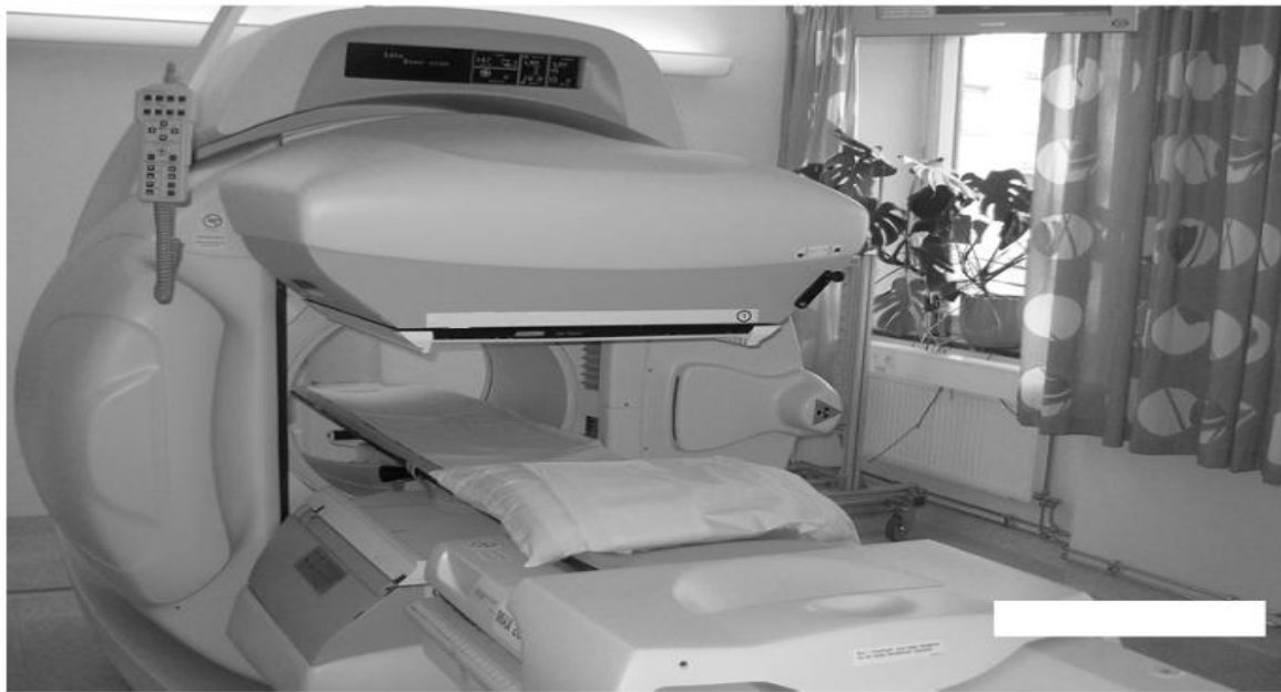
Figure 1: A gamma camera with capability to acquire planar whole-body and tomography images
