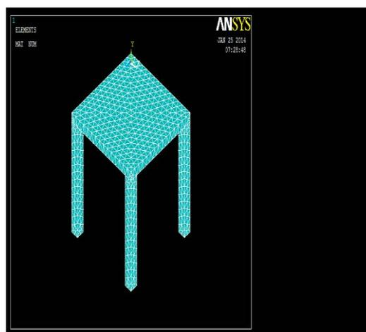
Figure 1: FEA model of TABLE built in ANSYS 12.
