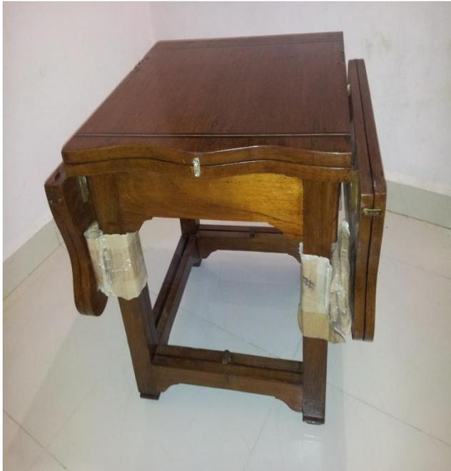
The table shown in the above image is manufactured by using the above described mechanisms which is made by using brass and teak wood with the help of cutting machine, hacksaw, planner etc. And hence the table can transform into various forms.
