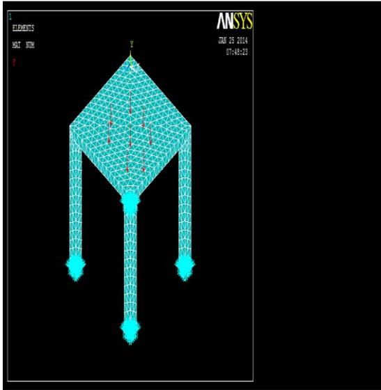
Figure 2: FEA model with boundary condition
