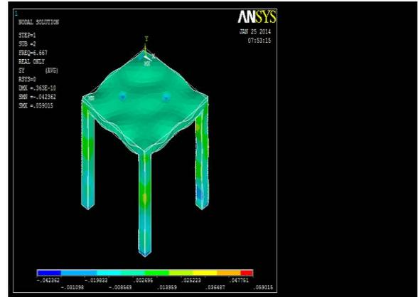
Figure 5: FEA model with y-direction displacement
