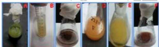
Figure 2: The conversion of silver nitrate to nano silver by Aspergillus flavus (A- in potato dextrose broth, B- cell free filtrate, C- cell free filtrate after addition AgNO 3 ) and Fusarium sp. (D- in potato dextrose broth, E- cell free filtrate F- cell free filtrate after addition AgNO 3 )
