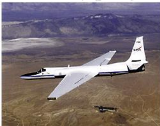
Figure 1: An ER – 2 uses LASE to take measurements of the atmosphere
