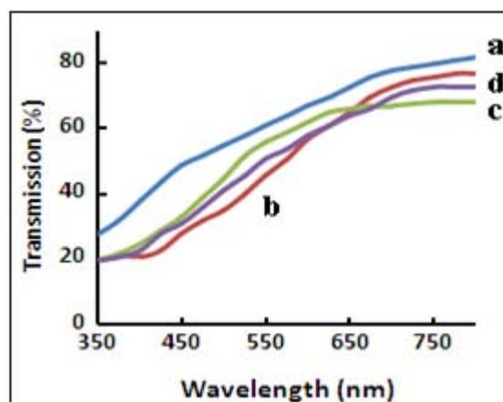
**Figure 1:** Transmission versus wavelength of as deposited thin films prepared at different substrate temperature a) 250°C b) 275°C c) 300°C and d) 325°C
