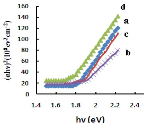
**Figure 2:** The graph between  $(\alpha h\nu)^2$  versus  $h\nu$  of as deposited thin films prepared at different substrate temperature a) 250<sup>0</sup>C b) 275<sup>0</sup>C c) 300<sup>0</sup>C and d) 325<sup>0</sup>C
