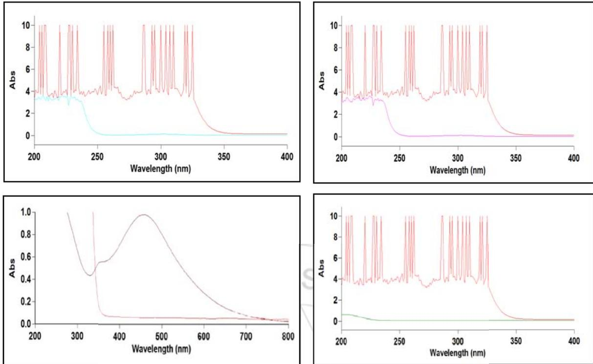
UV-visible absorption spectras showing AgNO<sub>3</sub> metal salt reduction by the treatment of root extracts of *Croton sparsiflorus* against normal AgNO<sub>3</sub>.
