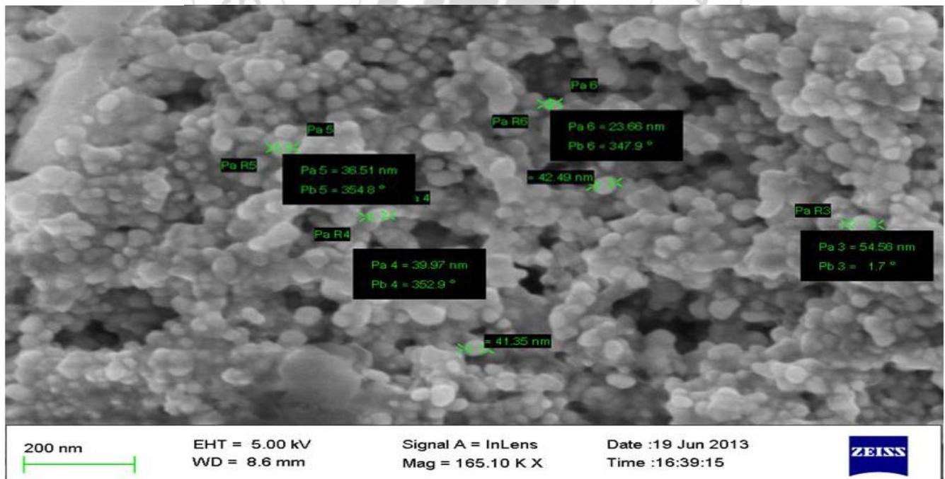
**Figure 2:** Scanning electron microscopic (SEM) studies of silver nanoparticles
