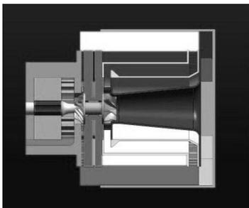
**Figure 1:** Micro Turbine with 20mm rotor diameter and Piezoelectric Diaphragm
