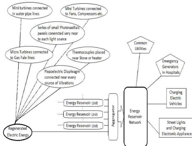
**Figure 3:** Schematic for Implementation of Energy Regeneration and Energy Reservoir Network
