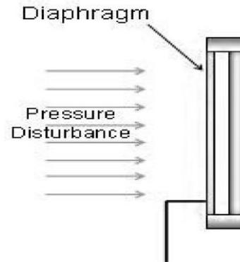
**Figure 2:** Piezoelectric Diaphragm
