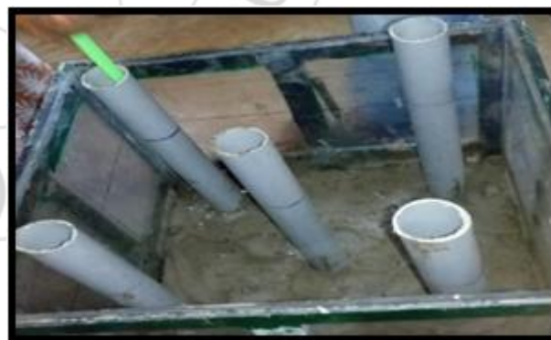
Figure 1: Lime pile installation during at laboratory
