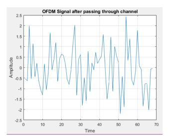
FFT is performed after passing through AWGN channel (as shown in 3.) and 2 bit IQ from Symbol de-mapper and this generates output bits (as shown in 4.)
