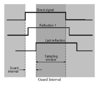
There are further advantages of the distribution of the data across multiple carriers. Only a few carriers are affected by the nulls caused by multi-path effects or interference on a given frequency while the remaining ones are received correctly. Almost all the data is reconstructed by using errorcoding techniques.
