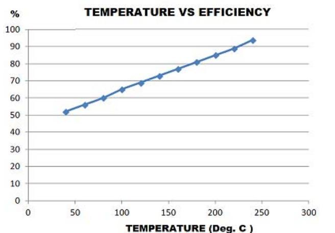
**Figure 8:** Temperature vs. Efficiency
