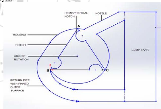
**Figure 1:** The detailed View of rotary engine.
