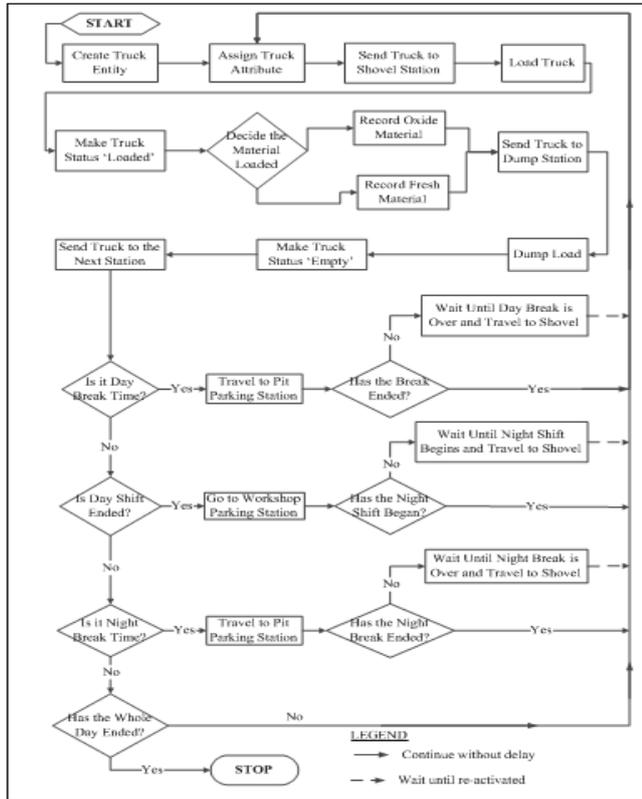
**Figure 1:** Conceptual model of shovel-truck system
