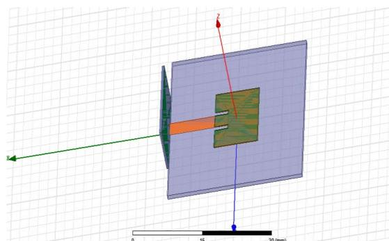
Figure 3: PAni-PTsA+MWCNT patch antenna
