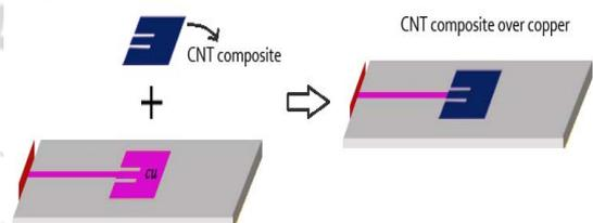
Figure 1: Typical structure of Nano composite thin film over the copper patch antenna
