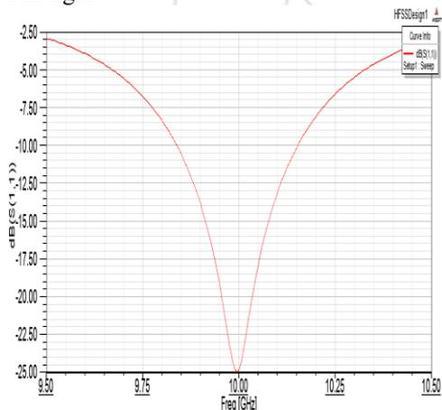
**Figure 7:** Simulated S11 of PANi-NSA with MWCNT patch antenna
