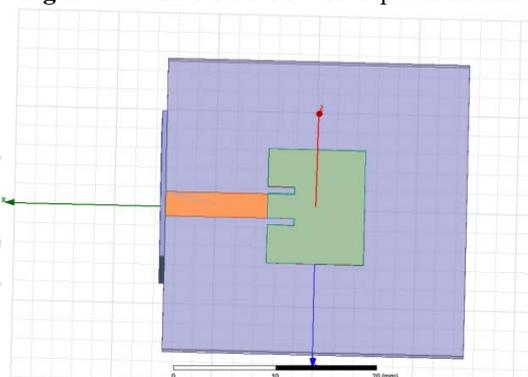
Figure 4: PAni-NSA + MWNT patch antenna
