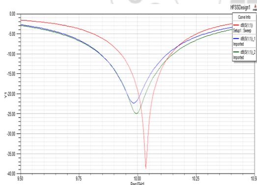
**Figure 11:** Bandwidth (BW) enhancement of MWCNT composite antennas compared to standard antenna. For (*PAni-PTsA*) MWCNT composite, 28.4% larger BW (Blue line); for MWCNT(*PAni-NSA*) composite, the BW is 31.2% larger (Green line) than the standard Microstrip antenna (red line).
