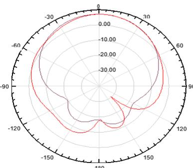
**Figure 10:** Simulated radiation pattern of PANi-NSA with Patch antenna MWNT patch antenna
