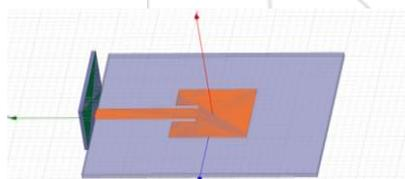
Figure 2: Single Element modelled in HFSS (Standard antenna)
