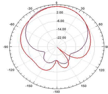
**Figure 8:** Radiation pattern of conventional patch antenna, Gain (dB)
