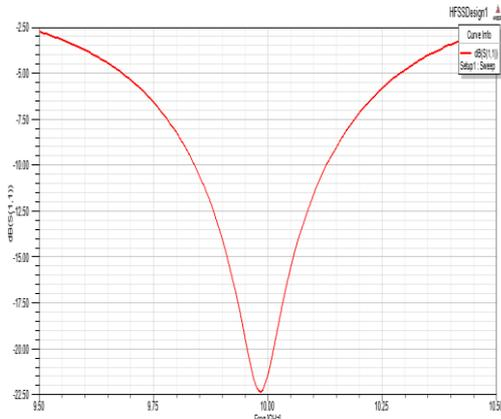
**Figure 6:** Simulated S11 of PANi-PTsA with MWCNT patch antenna
