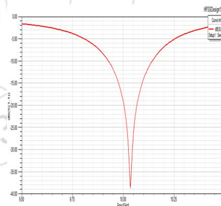
Figure 5: simulation of S11 [dB] conventional antenna
