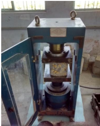
Figure 2: Compressive Strength Test
