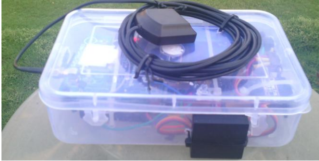
Figure 5.1: Authentication Locking and Tracking Unit
