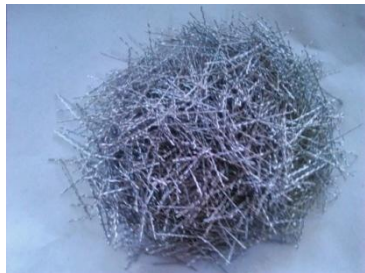
Figure 1: Crimped steel fibre
