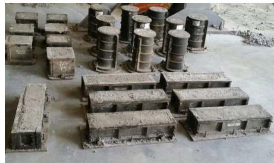
Figure 2: Casting of Specimens
