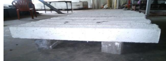
Figure 4: Beams after white washing
