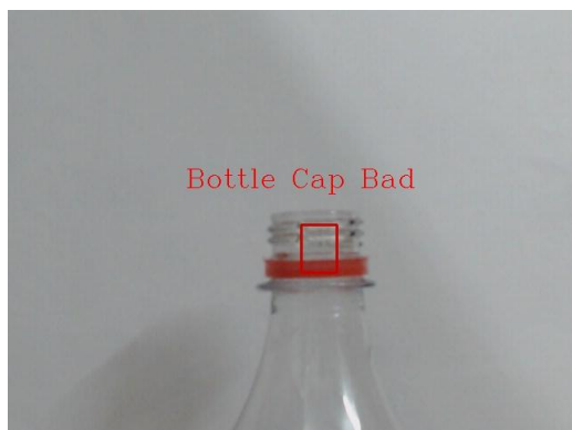
Figure 11: Presence Absence Result of Bottle with missing cap
