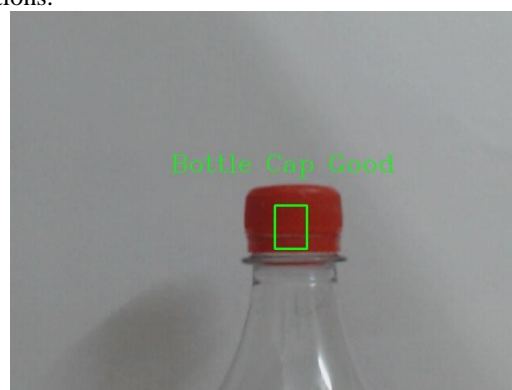
Figure 8: Presence Absence Result of Bottle with Good Cap
