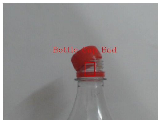
Figure 10: Presence Absence Result of Bottle with Bad Cap
