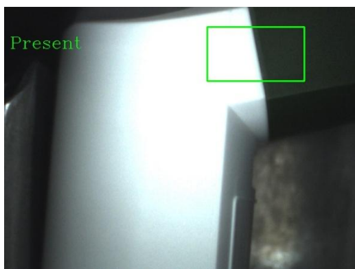
Figure 6: Inhaler Spray cap Presence-Absence Result
