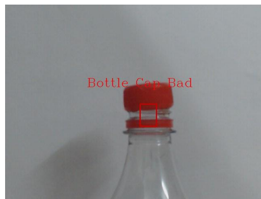
Figure 9: Presence Absence Result of Bottle with Bad Cap
