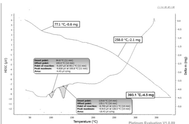
**Figure 2: TG/HDSC Thermogram of L1-Pd**
