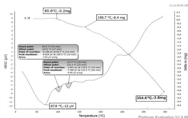
**Figure 5: TG/HDSC Thermogram of L2-Pd**
