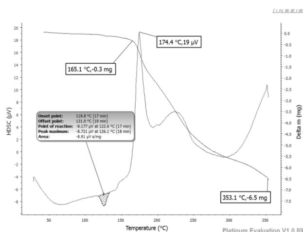
Figure 11: TG/HDSC Thermogram of L3-Ag
