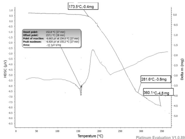
Figure 10: TG/HDSC Thermogram of L3-Ni
