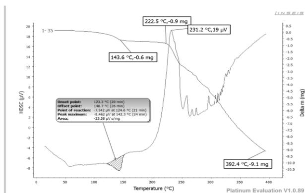
**Figure 1: TG/HDSC Thermogram of L1**
