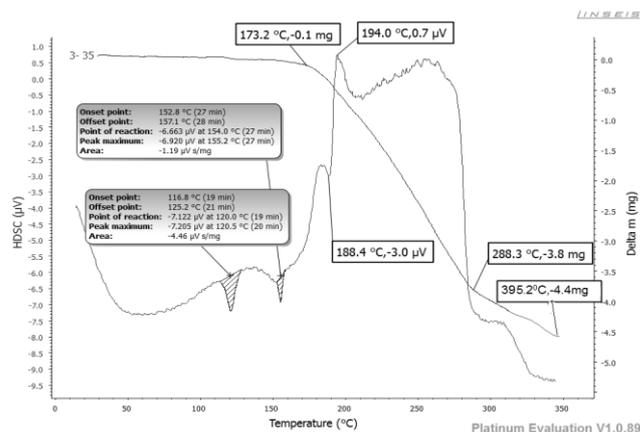
**Figure 3: TG/HDSC Thermogram of L1-Ag**
