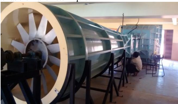
Figure 1: Lowspeed subsonic wind tunnel
