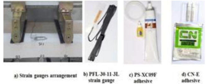
Figure 9: Strain gauge type, Arrangement, and Adhesive materials
