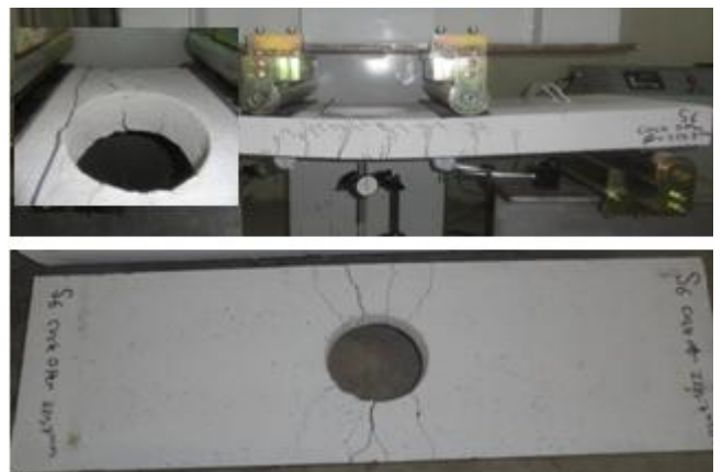
Figure 38: Crack pattern of specimen S6
