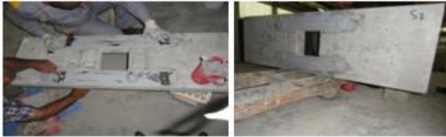
Figure 4: Making holes in RC slabs
