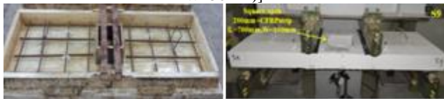
i:S9 [Square opening (200 mm) + CFRP strip (L=700mm, W=100mm)]
