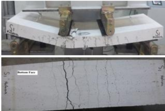
Figure 33: Crack pattern of specimen S1 (without opening)
