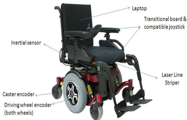
Figure 3(a): An electric-powered wheelchairs to detect hazardous terrain. (Barb Ruppert, TATRC science and technology writer, 2015)
