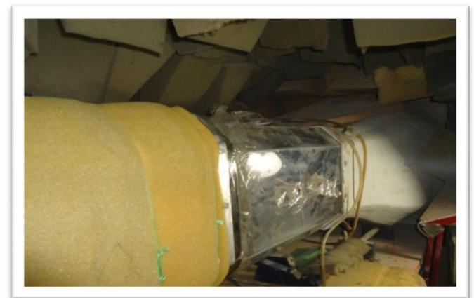
Figure 1: The anechoic chamber photograph for wind tunnel without cylinder.
