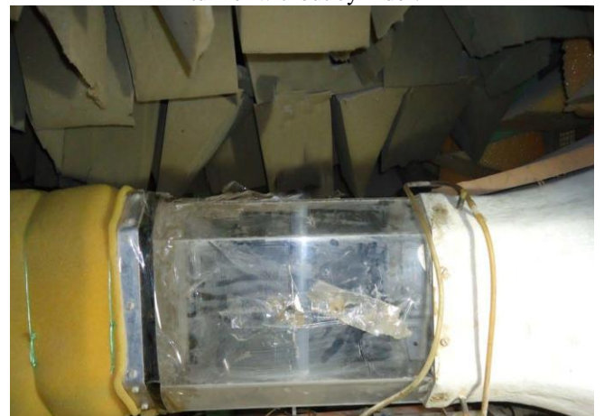
Figure 2: Photographic picture of the used test section for wind tunnel with cylinder.
