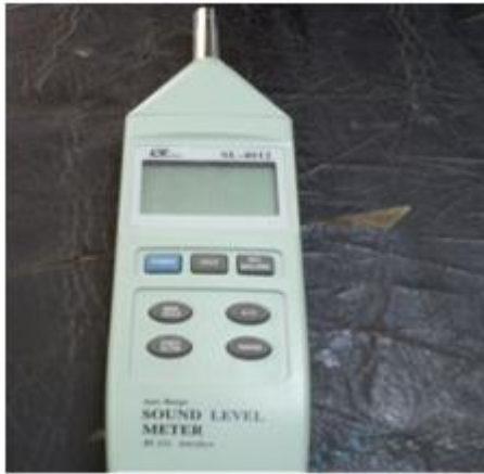
Figure 3: Photograph of sound level meter
