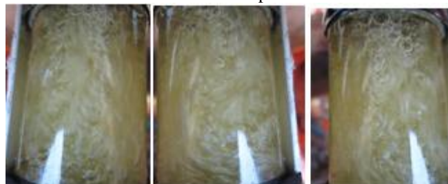
Figure 3: The actual flow pattern of reactant in novel OFR
