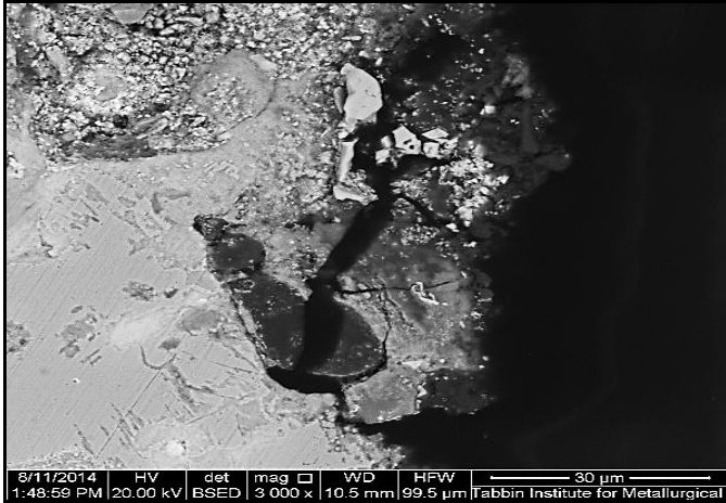
Figure 7: SEM ex., for a cross section of the Camel no. A shows lead globules (lighter areas), cracks and distorting alloy (3000x).
