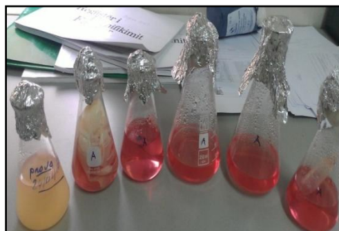
Photo 3: Products irradiated with dose 21 kGy
