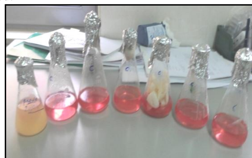
Photo 2: Products irradiated with dose 27 kGy
