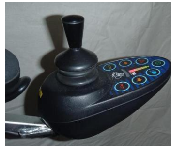
Figure 3: Typical Joystick for Wheelchairs
