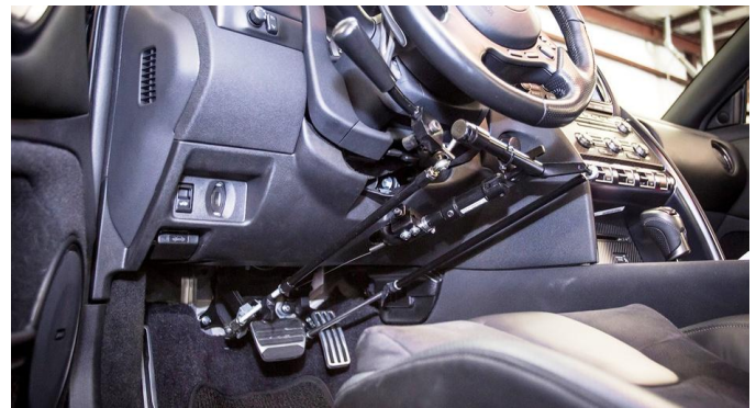
Figure 9: Modified controls of car [11]
