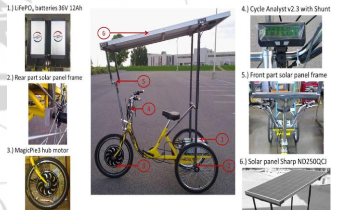
Figure 7: Solar-powered tricycle end design [6]
