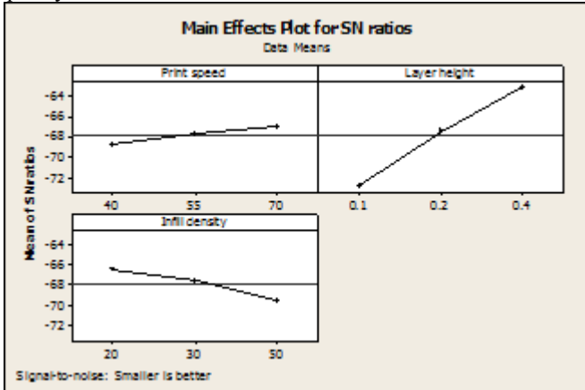
Figure 4: S/N Effects of process parameters on build time
