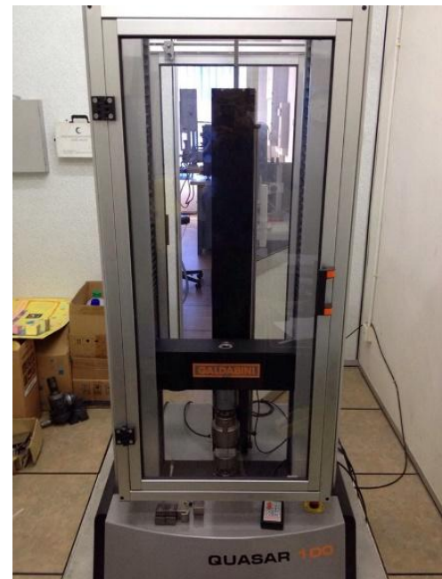
Figure 4: Universal Testing Machine (UTM) for Compression Test
