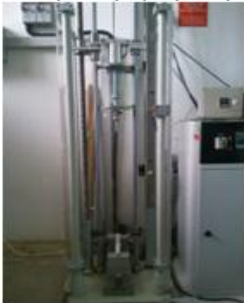
Figure 2: Drop-weight Tower for Drop-height Impact test
